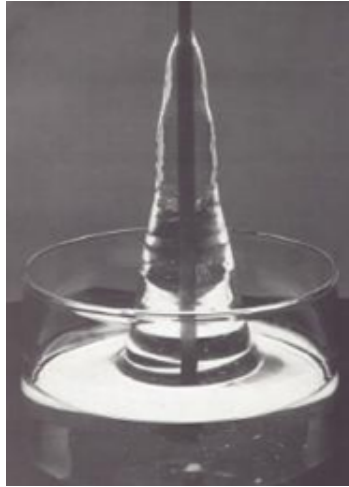
Figure 2.21: Rod climbing effect of a viscoelastic fluid. Source.: Barnes et al. (1989)
